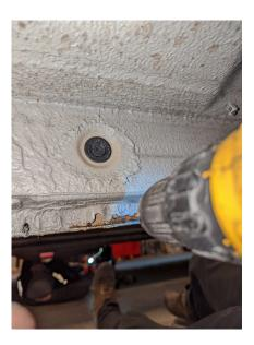
3. Mount the first bracket using the provided ¼" bolts and nuts.
