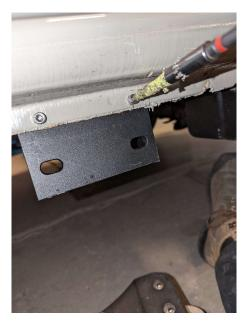
4. Mount the Nerf Bar hoop to both brackets to set the distance between bracket 1 and 2.
