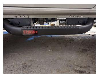
7. Position the passenger bracket as far forward, like shown in the picture.
