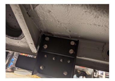
Once you've installed the first bracket mount your Nerf Bar hoop to both brackets to set the distance between both brackets.
