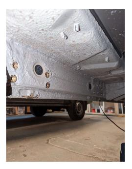
6. Mount brackets back on and attach your nerf bar hoops to the brackets.
