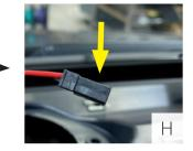
• Repeat this for the connector of the Jehnert Center crossover (fig. G/H) so that the connection fits between the crossover and the factory connection cable.
