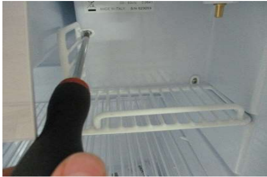
7. Unscrew the grid (2 screws)
