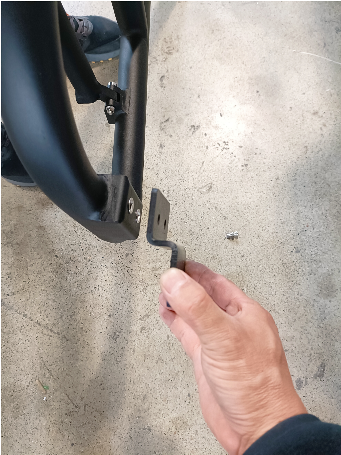
Picture 5: This image illustrates how the mounting tab should be attached to the tire ladder rack.
