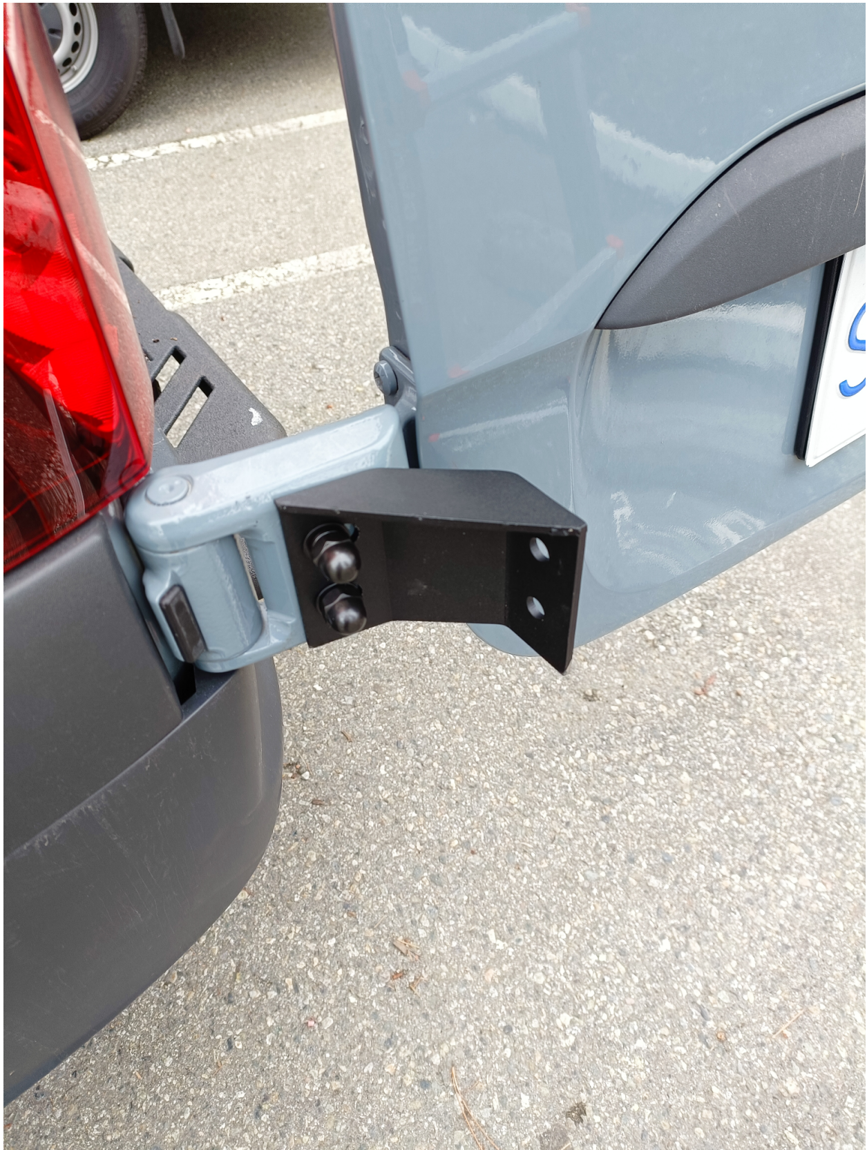
Picture 4: Here's the outside view of the lower hinge with the bracket installed.
