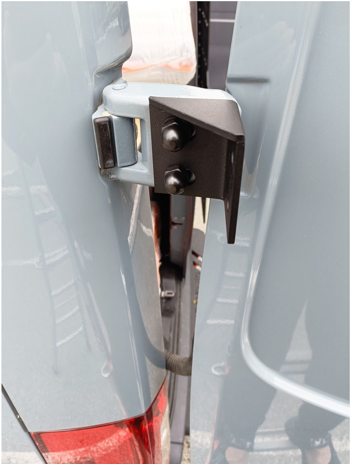
Picture 3: Here's the outside view of the upper hinge with the bracket installed.
