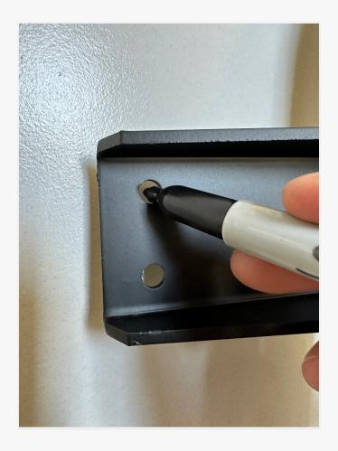
Step 3: Drill holes on the rear door hinges using the marked locations. Be sure to apply rust-proofing solution to the drilled holes to prevent corrosion.
