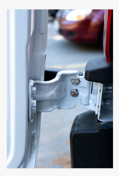
Step 6: Refer to the provided picture to mark the holes that need to be drilled through the rear door, then drill the holes.
